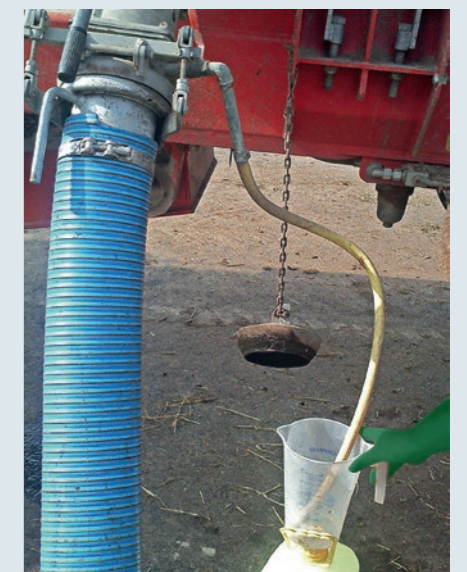
Addition via bypass
